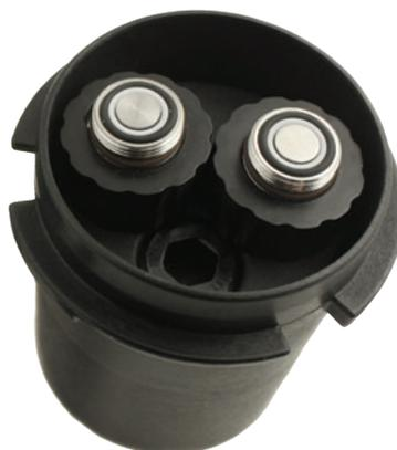
Well Cap with Two Levellogger Direct Read Cables Installed (one additional access hole available for monitoring)
