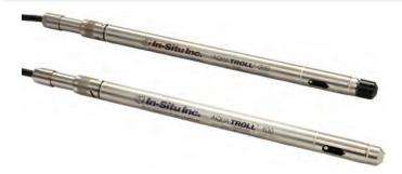
Conductivity measurements can be used to characterize water quality changes relative to a baseline or to estimate the concentration of contaminants. The In-Situ® Aqua TROLL 100 and Aqua TROLL 200 Instruments measure and log conductivity and temperature. The Aqua TROLL 200 adds water level logging.
